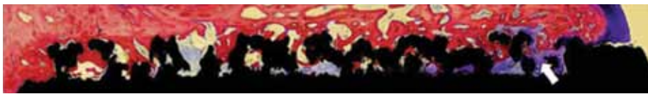
Figure 1: Pictured above is a 75µm section view from a weight-bearing Ovine study showing bone ingrowth into the Tesera trabecular structure at 12 weeks. 1
